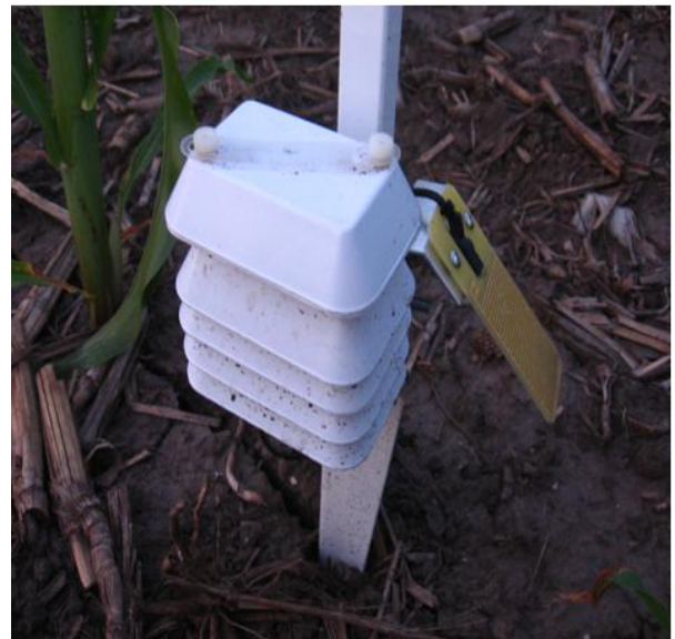
Site-specific environmental conditions influence plant disease and pests. Above is a mini-weather station at the Illinois PFR Center. This unit is a data logger that measures leaf wetness, temperature and humidity and is made by Spectrum Technologies located in Naperville, Illinois.
